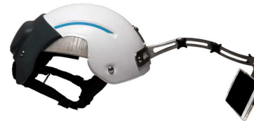
Fig. 6 : Final smartphone funduscopy device (lateral view)
